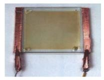
Electrochromic window in its lightened state (Image Source: NREL)
