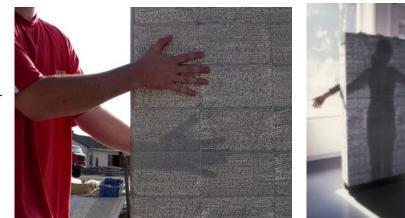
Light Transmitting Concrete Image Source: LiTraCon™ (www.litracon.hu)
