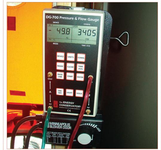
This gauge for the blower door test tells the user exactly how leaky the house is.
