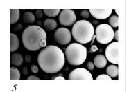
**Fly-Ash Concrete** - Fly-ash concrete is used for the wall and floor panels of Melrose II. Fly ash is a common substitute for cement, an energy-intensive material typically used in concrete. Fly ash is a byproduct of coal burning and comes from the impurities in the coal that evaporate in the boiler and then condense into tiny glass spheres (5, 6). Fly ash is known as a "pozzolan" and reacts with hydrated lime, an unwanted byproduct of concrete, curing to produce additional cement-like gel.
