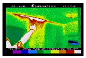
Infrared thermograph showing hot attic air being pulled into interior wall cavities (Florida Solar Energy Center photo)
