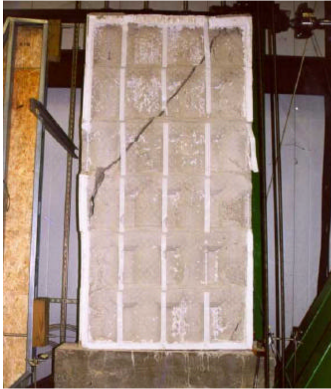
Figure 7 Failure Mechanism of Waffle No. 1 Wall Specimen
