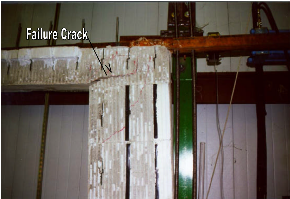
Figure 5 Failure Mechanism of Flat No. 3 Wall Specimen
