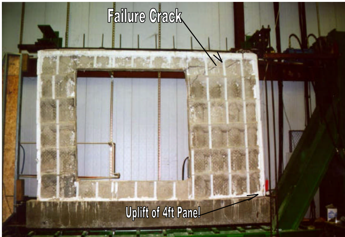
Figure 9 Failure Mechanism of Waffle No. 2 Wall Specimen
