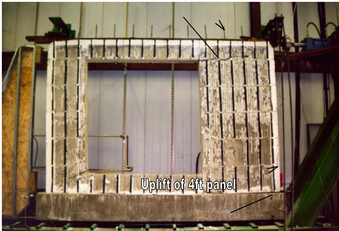
Figure 4 Failure Mechanism of Flat No. 2 Wall Specimen
