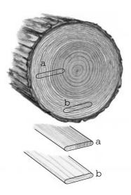
boards may check or crack as part of the natural weathering process. Weathering can be reduced by using a penetrating finish that contains a water repellent early in the finishing process. Allowing a deck to weather for a year opens the surface pores and permits the wood to accept more finish, but this weathering damages the wood. Research indicates that it is better to finish a deck as soon as it is dry (a few weeks after construction) and to refinish it in 2 years.
