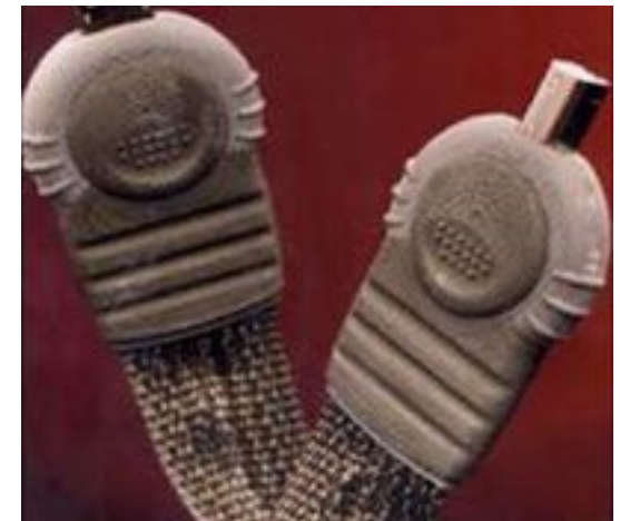
Electro-textile fabric with USB connectors Image Source: PATH ( www.pathnet.org )
