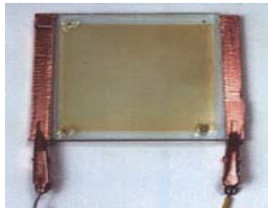
Electrochromic Windows in light & dark states (National Renewable Energy Lab)
