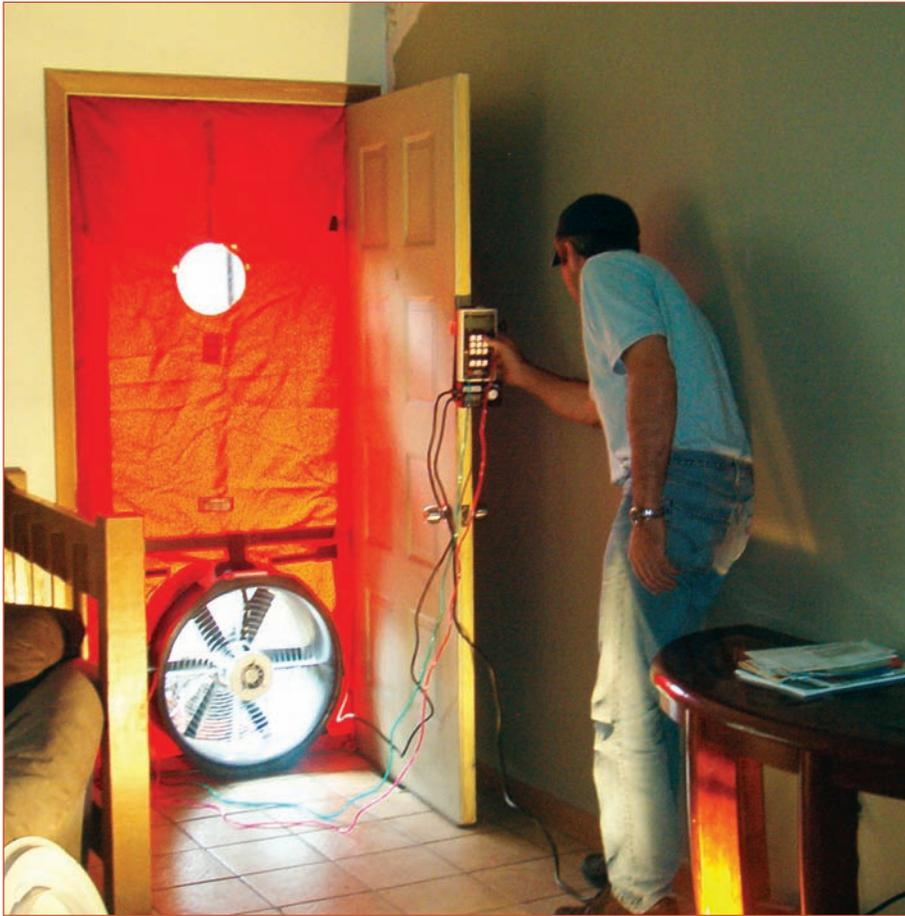
Building performance testing—which includes blower door testing and air infiltration testing—will determine whether a home’s HVAC system and building envelope are operating properly and where repairs and material upgrades are needed.
