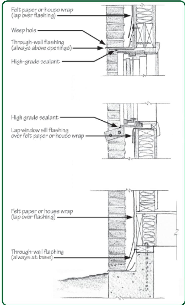
Figure 4.15 - Typical Brick Veneer Flashing Details
