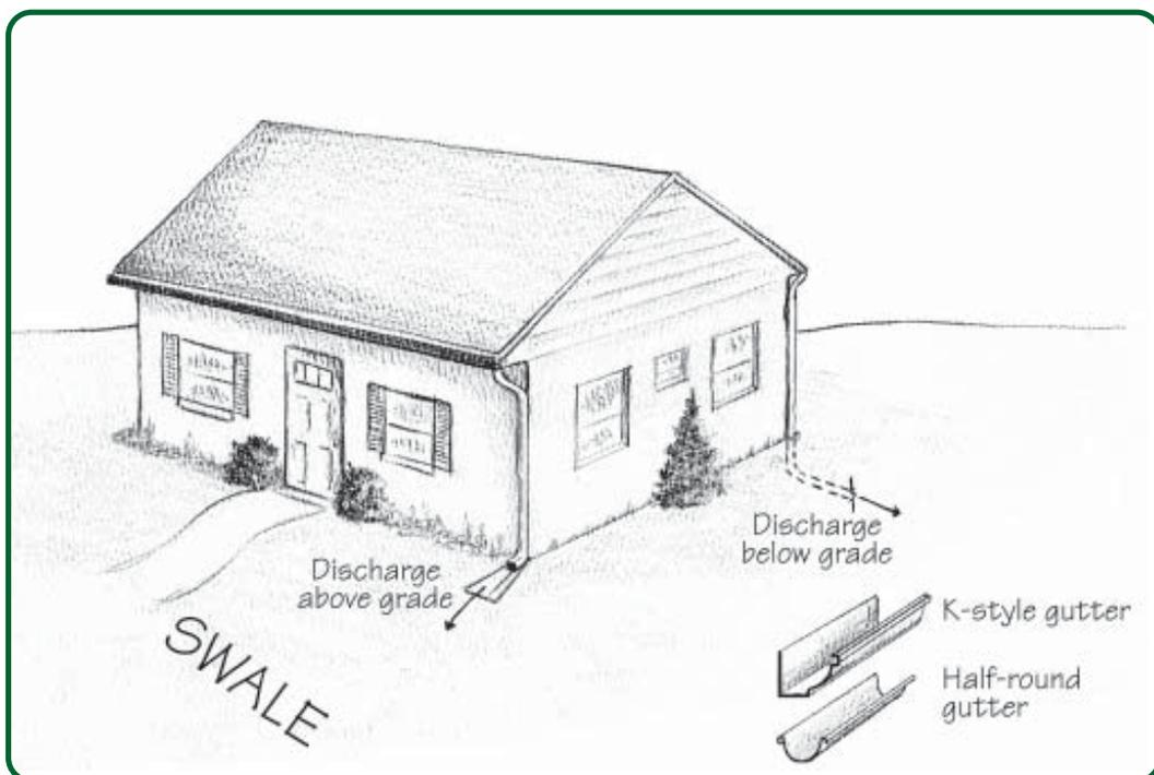
Figure 4.4 - Roof Gutters and Discharge Methods
