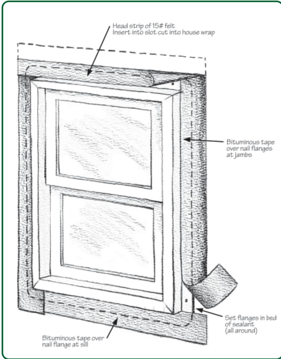
Figure 4.12 - Window Flashing for Severe Weather
