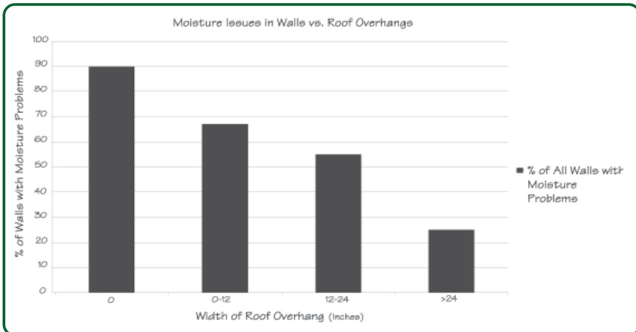
Figure 4.1 - Frequency of Moisture Problems in Walls of Selected Buildings in a Moist, Cool Climate
