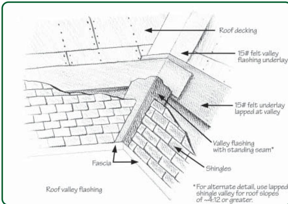
Figure 4.8b - Basic Roof Flashing Illustrations (continued)
