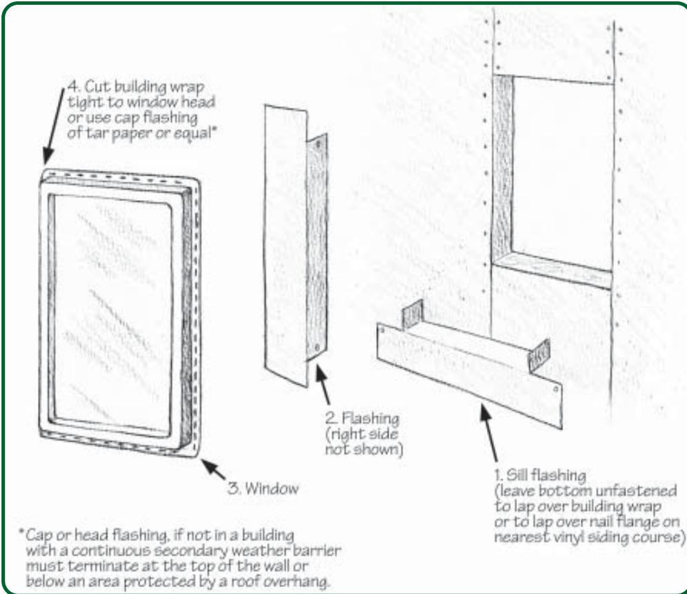
Figure 4.11 - Window Sill and Jamb Flashing Detail
