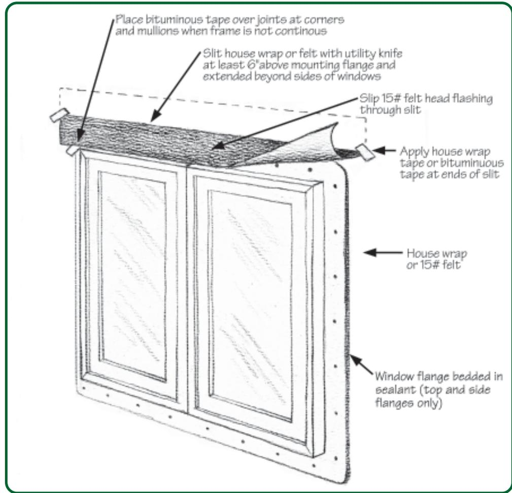
*Figure 4.10 - Window Flashing Illustration*
