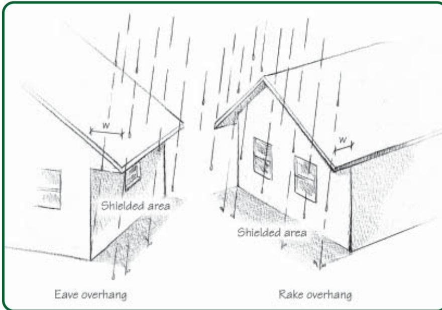
Figure 4.2 - Roof Overhangs
